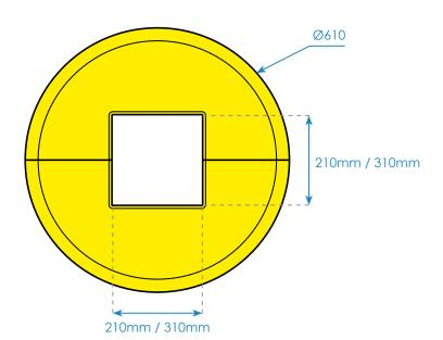
Each column protector is made from linear low density polythene (LLPE) Stress crack resistance; 550 hrs per ASTM D-1693 (110% LGEPAL) UV Stabilised (suitable indoors and outdoors)
